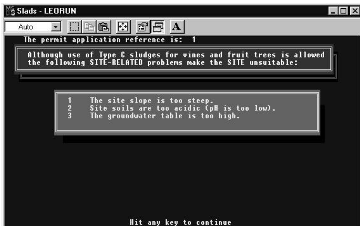
Figure 10: Issues which make the site unsuitable for sludge application.
