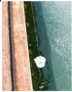
Use a clean bucket to collect water. Make sure not to scrape the bucket against the concrete wall when pulling it up.
