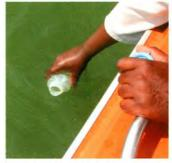
Collect the sample by lowering the bottle into the water, Perform a forward scoop motion if the boat is not moving.
