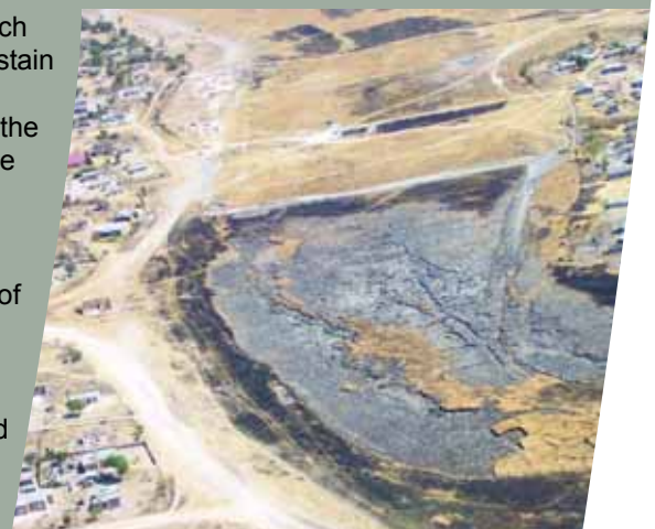
Burning peatland at Bodibe, near Mafikeng due to over utilisation of groundwater by local municipalities and farmers.
