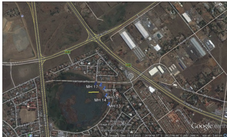
Figure 25: Blaauwpan, showing the line of manholes for the sewer that goes into the Elgin Street wetland just across the road to the North. The yellow lines is 100 m
